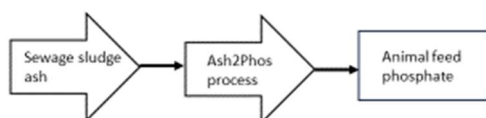
Figure 7: Steps in the pathway from sewage sludge ash to recycled phosphate for animal feed
