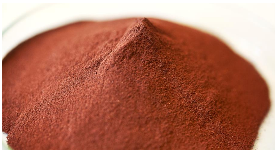
Figure 1. Dried silicate sand product with about 15 % wt. hematite, which give it a reddish brown colour (case 1; see the text below)
